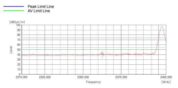
AV Detector: RBW: 1 MHz, VBW: 10 Hz (2 310 MHz - 2 390 MHz), Worst case (Low, Horizontal)
