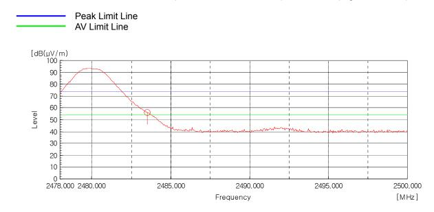
AV Detector: RBW: 1 MHz, VBW: 10 Hz (2 483.5 MHz - 2 500 MHz), Worst case (High, Horizontal)
