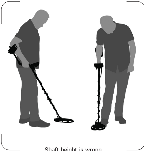
Shaft height is wrong
