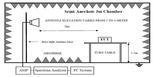
In Semi Anechoic Chamber (3m) Test Setup Diagram for Above 1GHz
