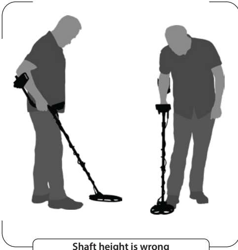
Shaft height is wrong
