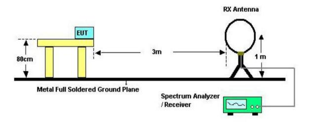
In Semi Anechoic Chamber (3m) Test Setup Diagram for 30MHz~1000MHz
