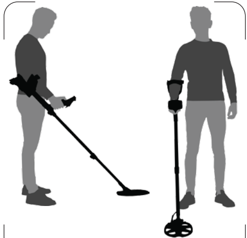
Shaft height is correct
