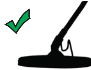
Correct search coil angle
