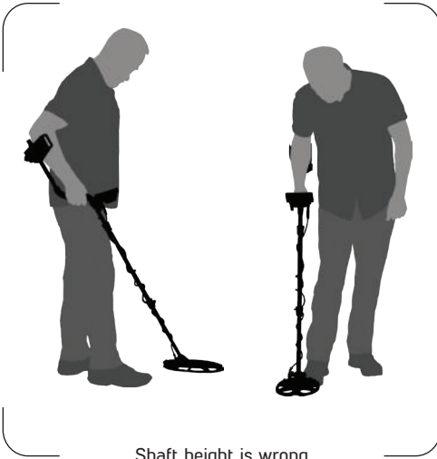
Shaft height is wrong
