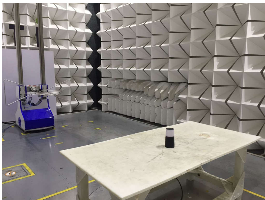
Radiated spurious emission Test Setup-2(30MHz-1GHz)
