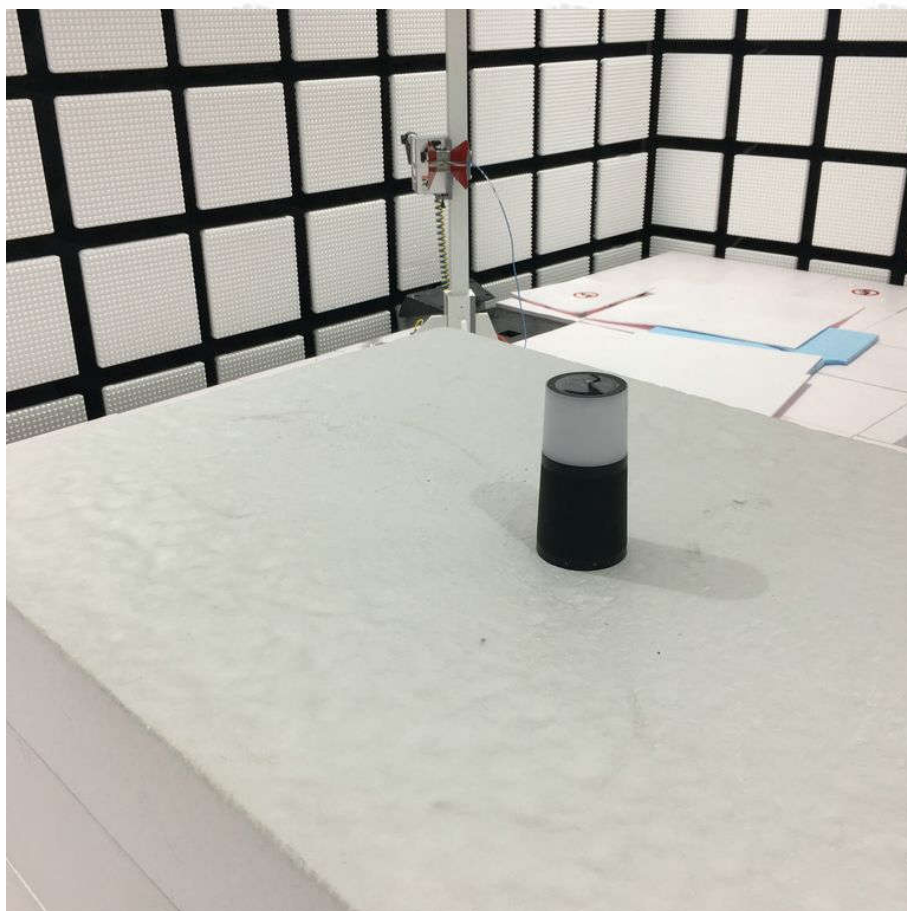
Radiated spurious emission Test Setup-3(Above 1GHz)
