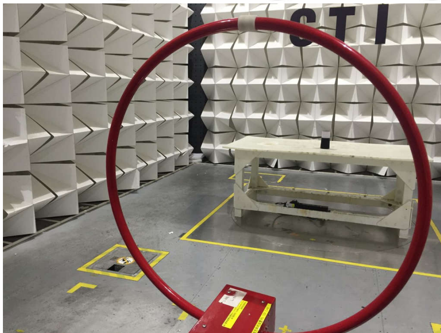
Radiated spurious emission Test Setup-1(Below 30MHz)
