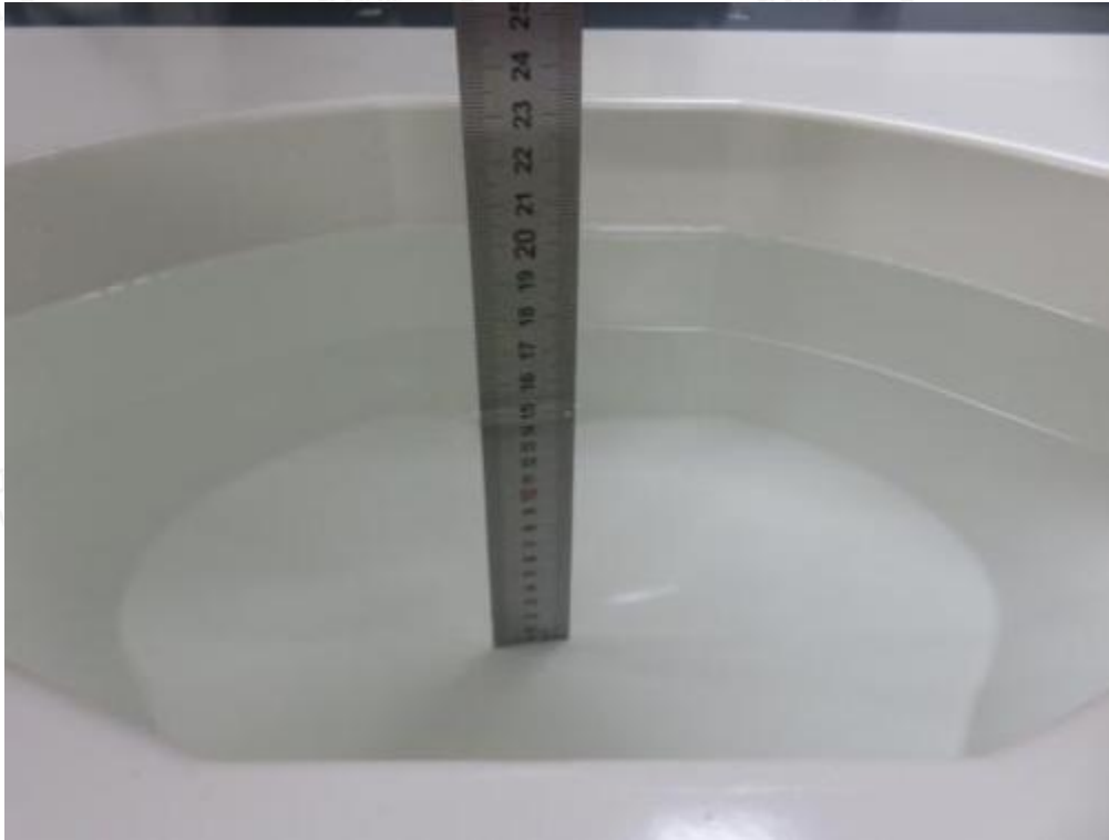
Photograph of the depth in the Head Phantom (2450MHz, 15.1cm depth)
