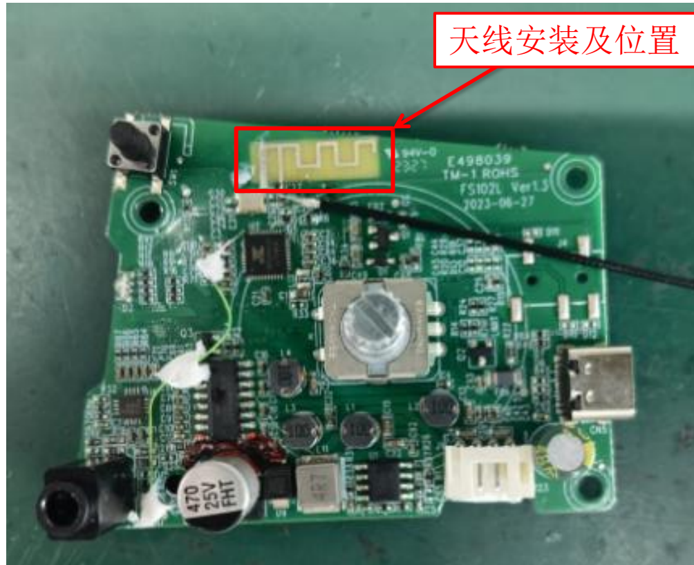
Antenna installation and location
