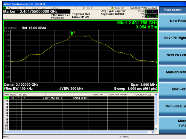
GFSK LOW CHANNEL, CARRIER LEVEL
