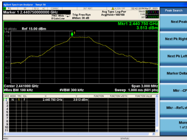
GFSK MIDDLE CHANNEL, CARRIER LEVEL
