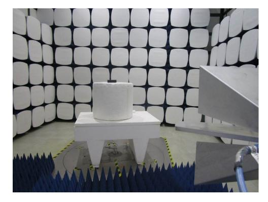
1.3 Radiated Spurious Emissions Test Setup
