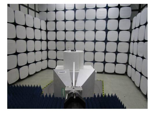
1.2 Radiated Spurious Emissions Test Setup
