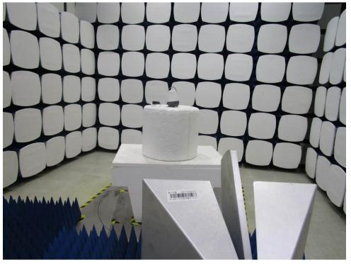
1.3 Radiated Spurious Emissions Test Setup
