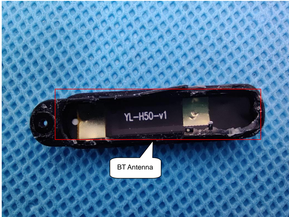
INTERNAL VIEW OF EUT (FIGURE 2)
