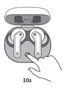
Press and hold the Multifunction Button for 10s or until the LED indicator flashes red 5 times. Upon completion, the earbuds will automatically enter Bluetooth pairing mode and the LED indicator will flash green. Master Reset is reserved for cases where users encounter issues while earbuds are in use or during situations such as:
