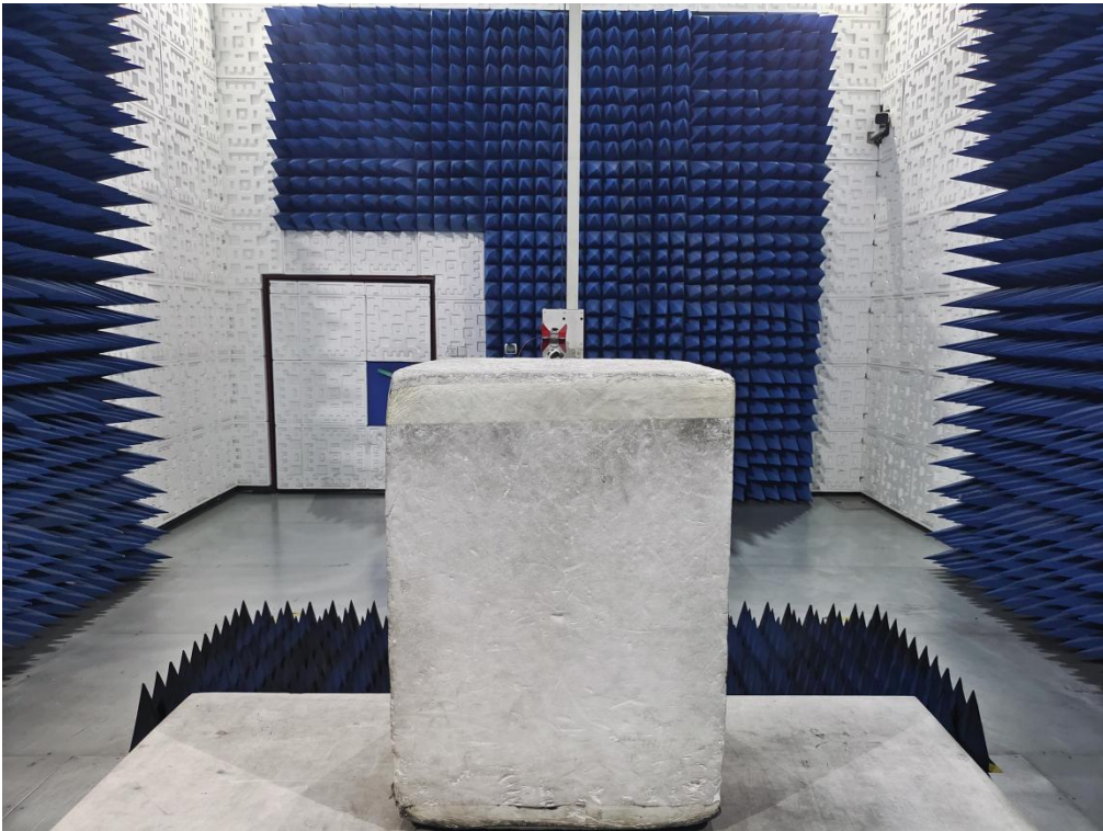
RADIATED EMISSION TEST SETUP ABOVE 1GHz
