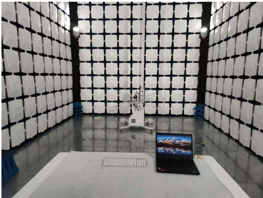
Blow 1GHz for radiated emission test setup
