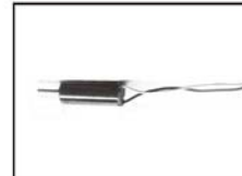
#4 Motor A with Red and blue wires (clockwise rotation)
