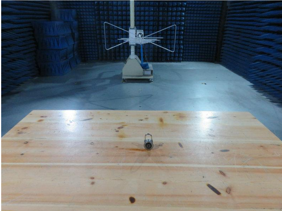
Photo of Radiation Emission Test
