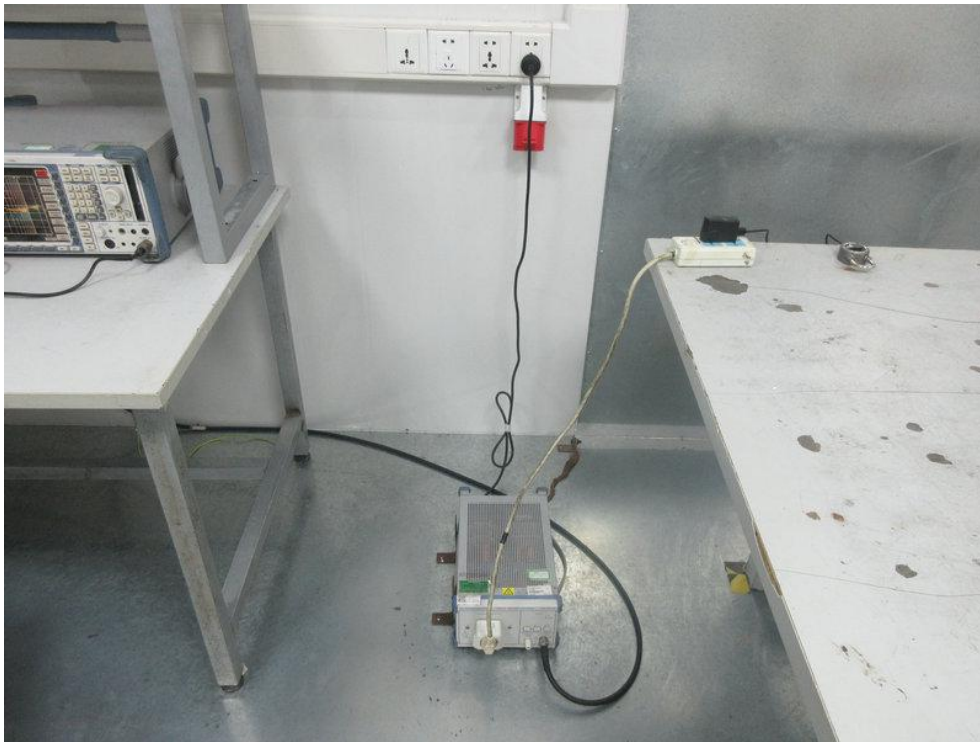
Photo of Power Line Conducted Emission Test
