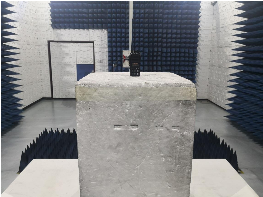
RADIATED EMISSION ABOVE 1G TEST SETUP
