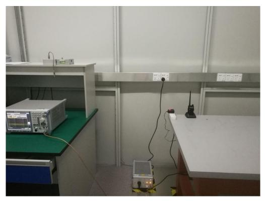
RADIATED EMISSION TEST SETUP
