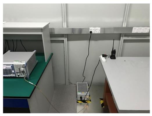
RADIATED EMISSION TEST SETUP
