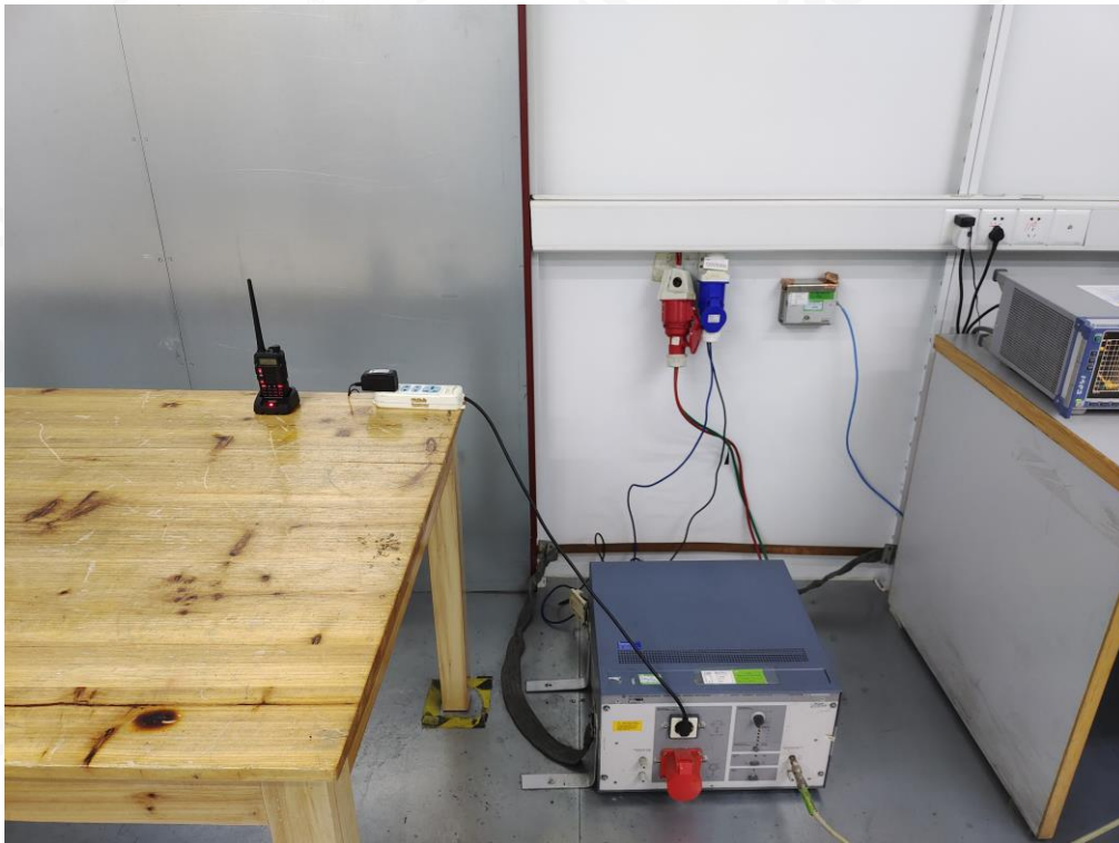
RADIATED EMISSION TEST SETUP-BELOW 1GHZ
