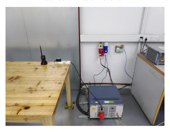
RADIATED EMISSION TEST SETUP-BELOW 1GHZ
