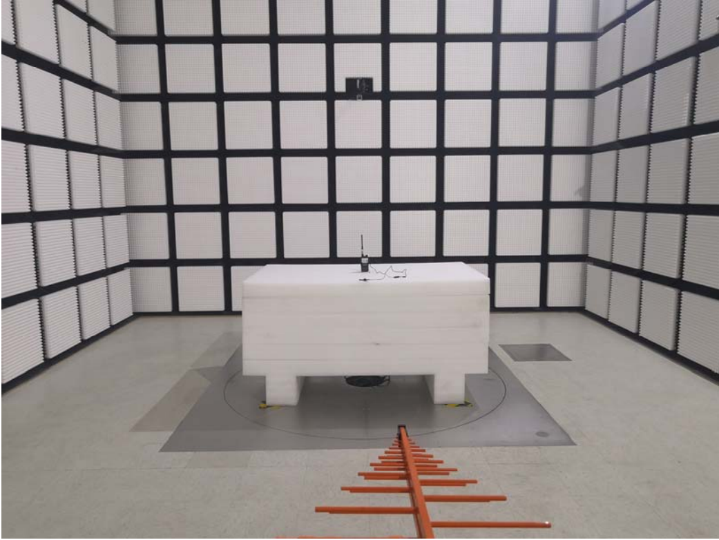
Radiated Emissions Below 1G View-TM4
