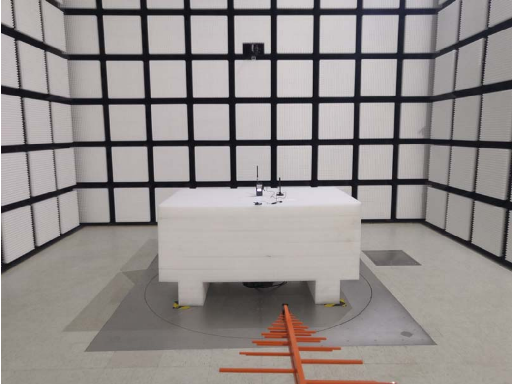
Radiated Emissions Below 1G View-TM4
