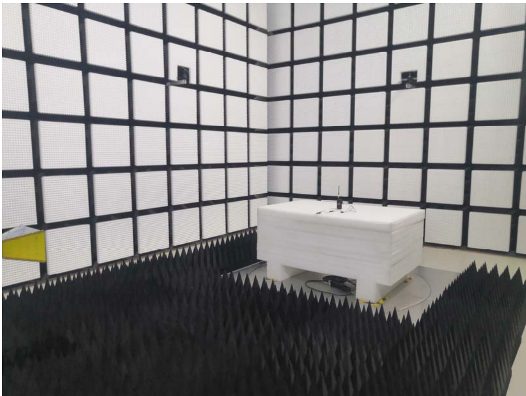
Radiated Emissions Above 1G View-TM4
