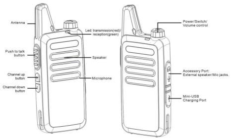
NOTE: Long press [Channel down] key to enter the monitoring state.
