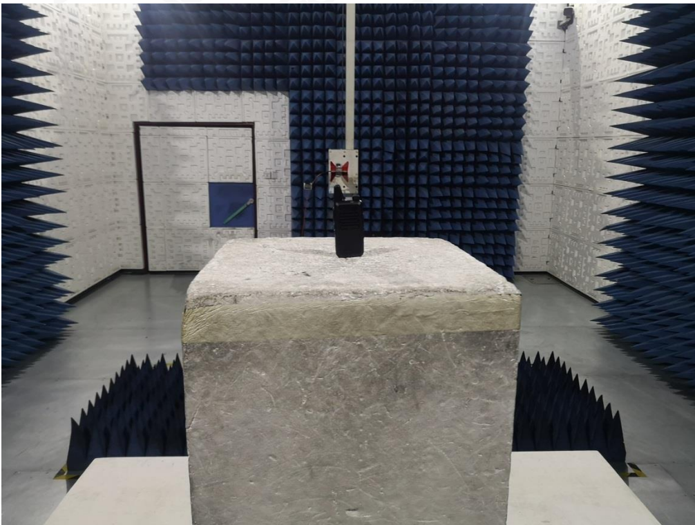
RADIATED EMISSION ABOVE 1G TEST SETUP
