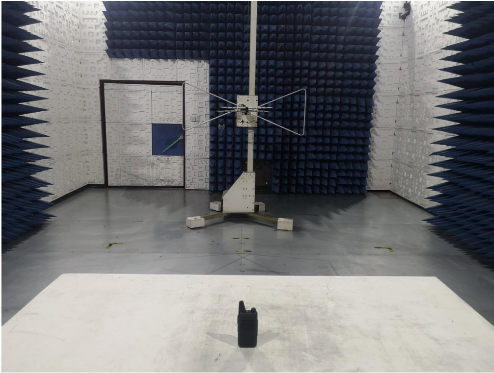
RADIATED EMISSION ABOVE 1G TEST SETUP
