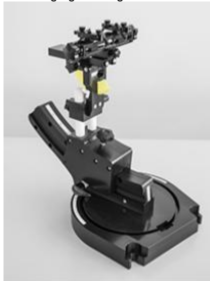
Device holder supplied by SPEAG
