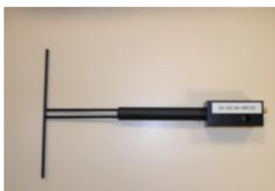
Figure 1 – MVG COMOSAR Validation Dipole
