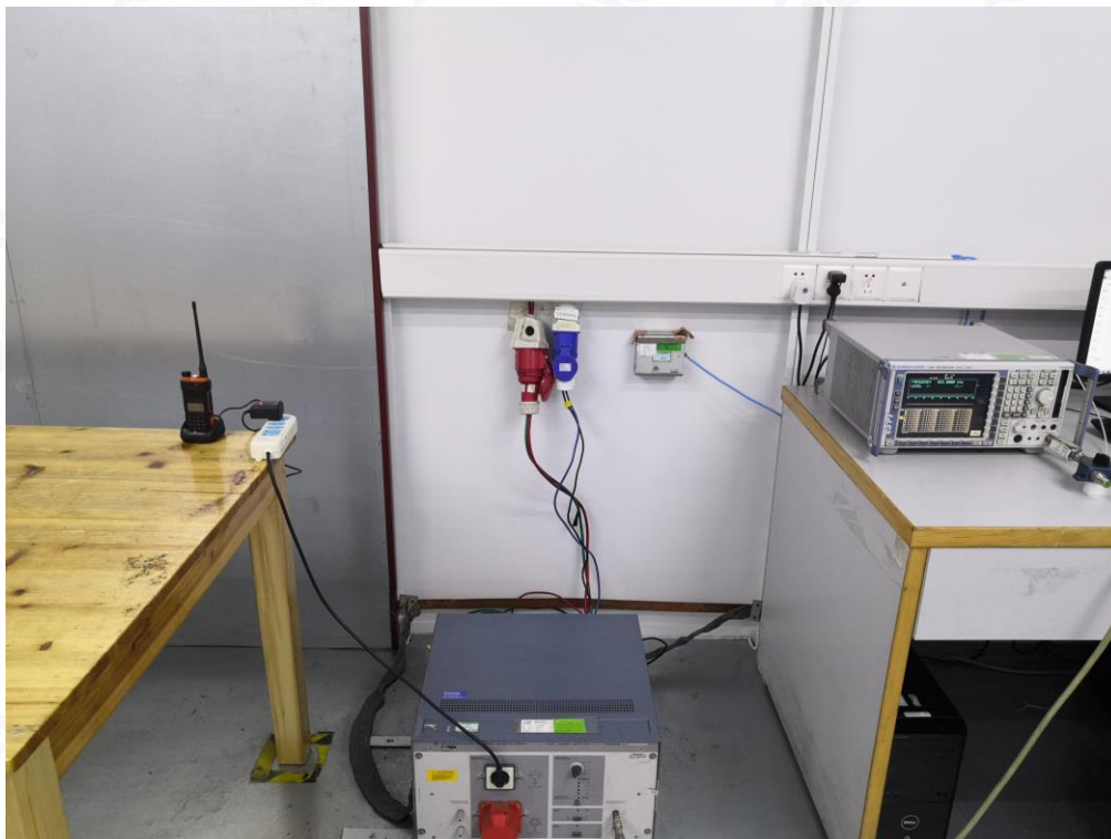
RADIATED EMISSION TEST SETUP-BELOW 1GHZ
