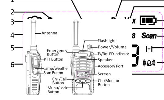
1. Channel(1-22)7. VOX (Off,1,2,3)2. Keypad Lock8. Battery Indicator3. Transmit Status9. CTC/DCS4. Receive Status10. NC5. Power High/Low11. Emergency(Off,1,2)6. Dual Channel Monitor12. Sub-Code(1-105)
