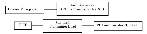
Setup Block Diagram for Audio Frequency filter:
