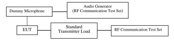
Setup Block Diagram for Audio Frequency filter:
