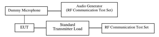
Setup Block Diagram for Audio Frequency filter:
