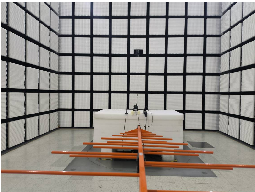
Radiated Emission Below 1GHz Rear View M2
