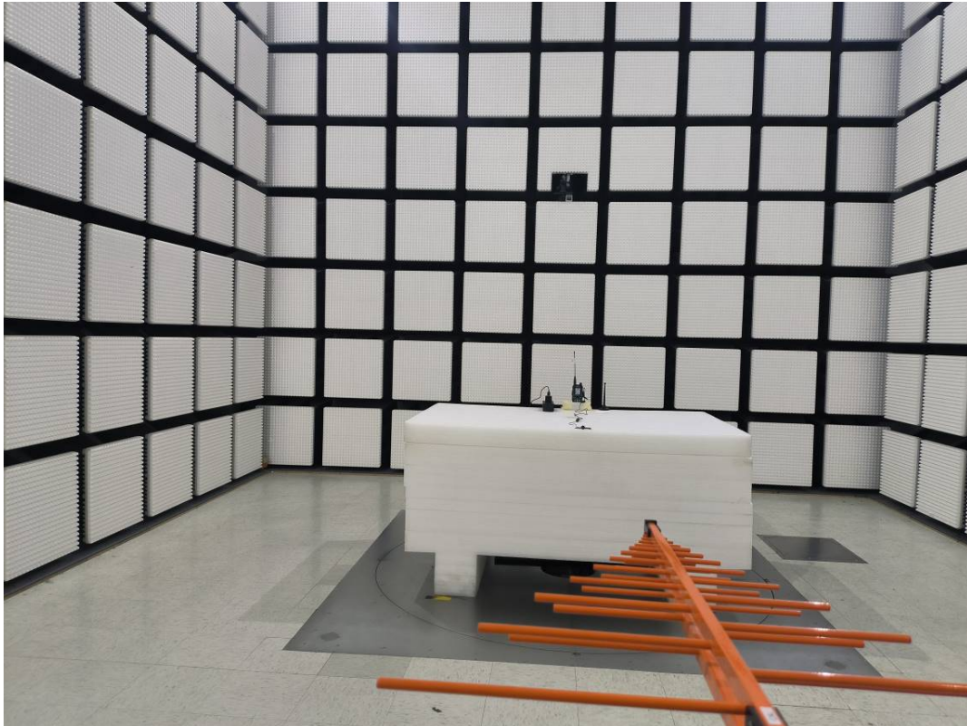
Radiated Emission Below 1GHz Rear View M2
