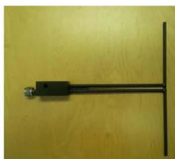
Figure 1 – MVG COMOSAR Validation Dipole
