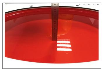
Liquid depth in the ELI Phantom(450MHz)
