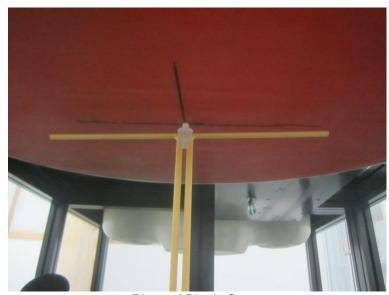
Photo of Dipole Setup
