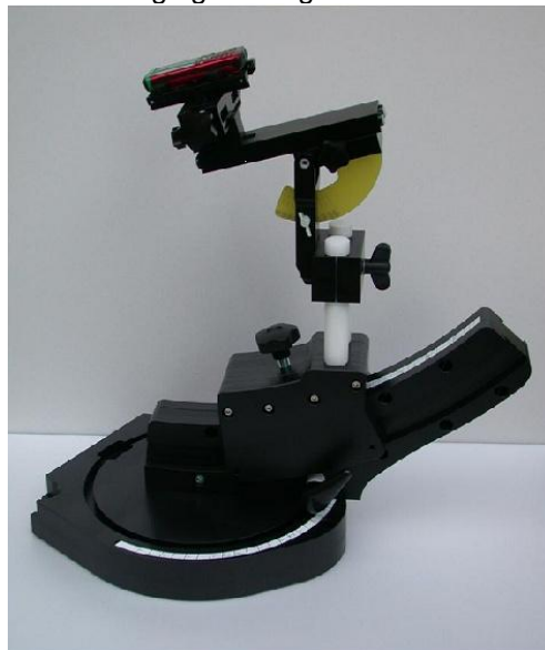
Device holder supplied by SPEAG
