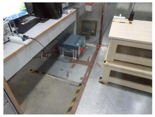
RADIATED EMISSION TEST SETUP
