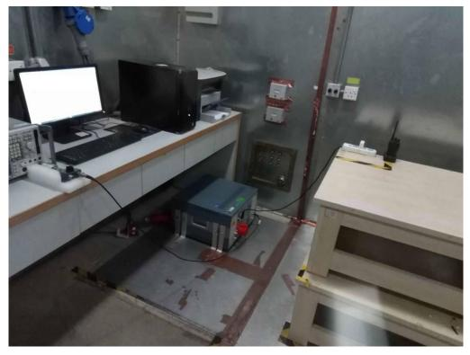
RADIATED EMISSION TEST SETUP
