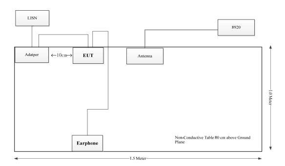
For Radiated Emission Test:
