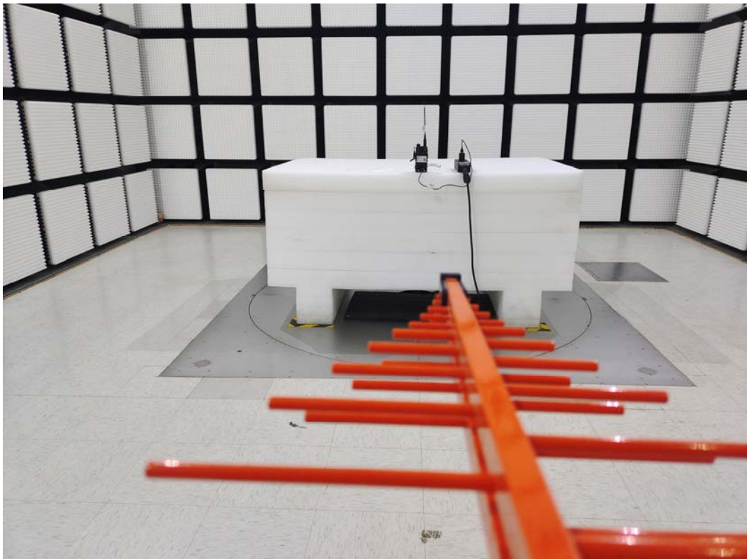
Radiated Emission Below 1GHz rear View M1
