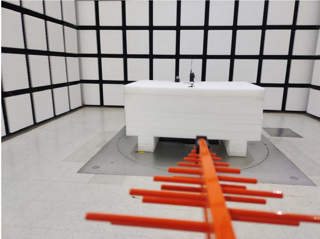
Radiated Emission Below 1GHz rear View M1
