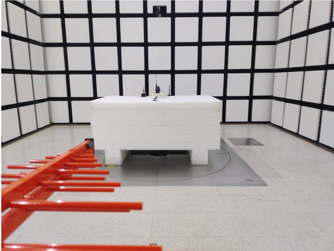
Radiated Emission Below 1GHz rear View M2
