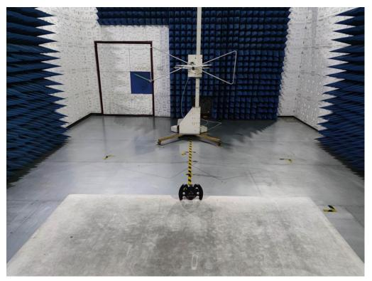
RADIATED EMISSION TEST SETUP ABOVE 1GHz
