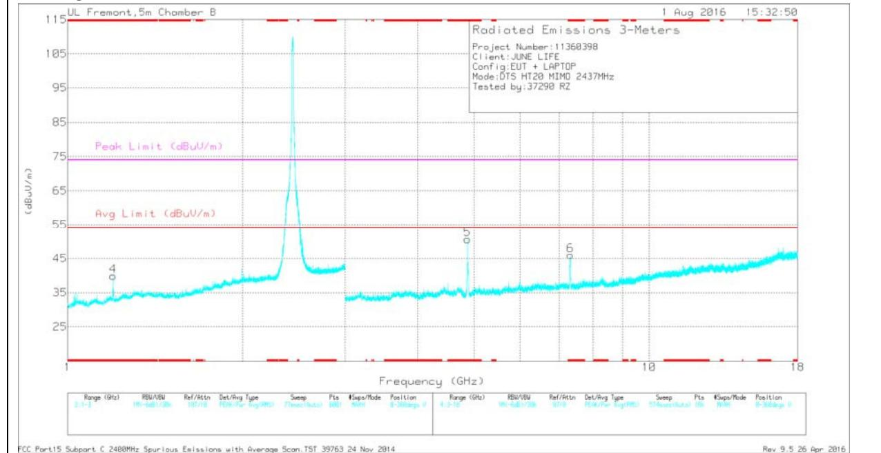
FCC Part15 Subpart C 2400MHz Spurious Emissions with Average Scan TST 39763 24 Nov. 2014
