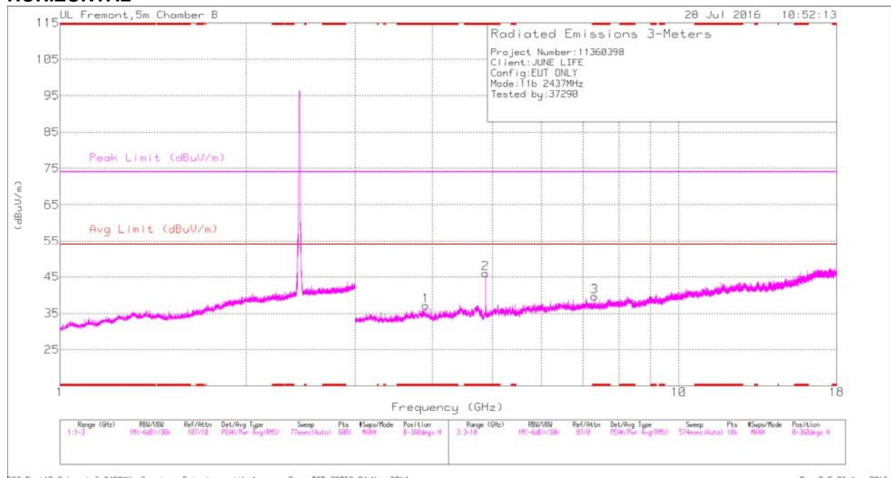
FCC Part15 Subpart C 2400MHz Spurious Emissions with Average Scan TST 39763 24 Nov 2014
