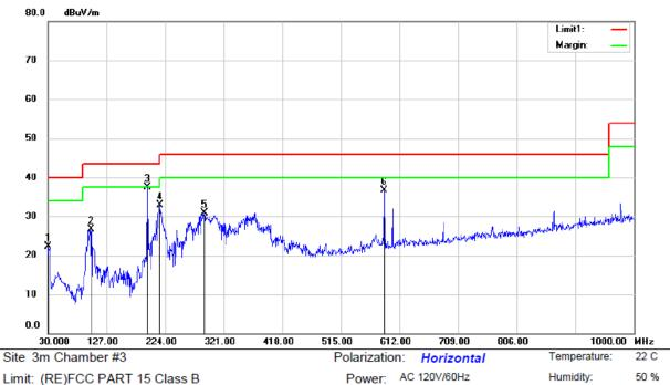
Limit: (RE)FCC PART 15 Class B Mode: 802.11a 5240MHz TX
