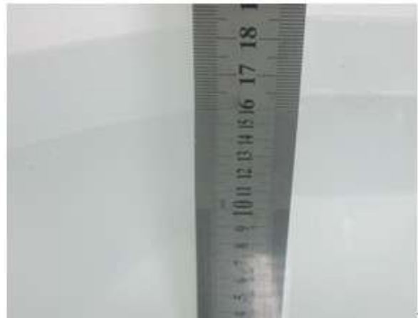
Liquid Height for Body SAR
