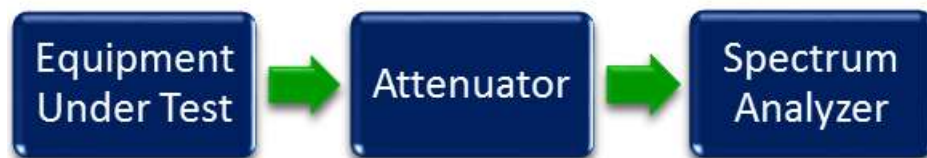
Figure 2. Occupied Bandwidth Test Setup
