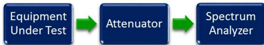
Figure 3. RF Power Test Setup
