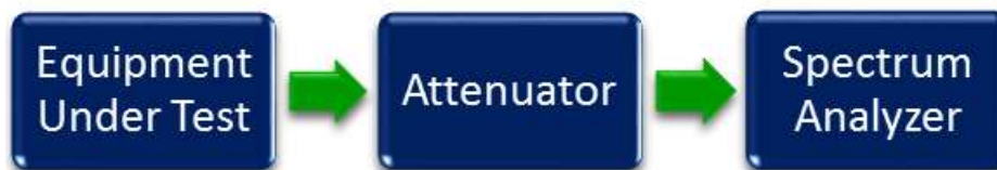
Figure 4. Conducted Spurious Emissions Test Setup
