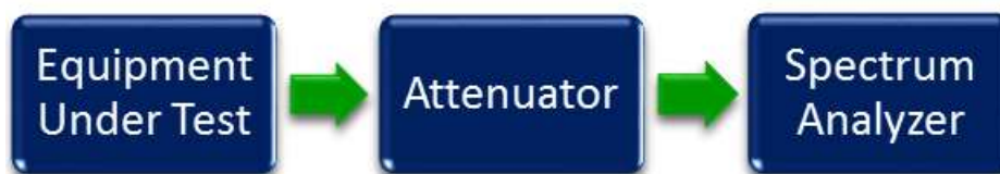
Figure 6. Band Edge Test Setup
