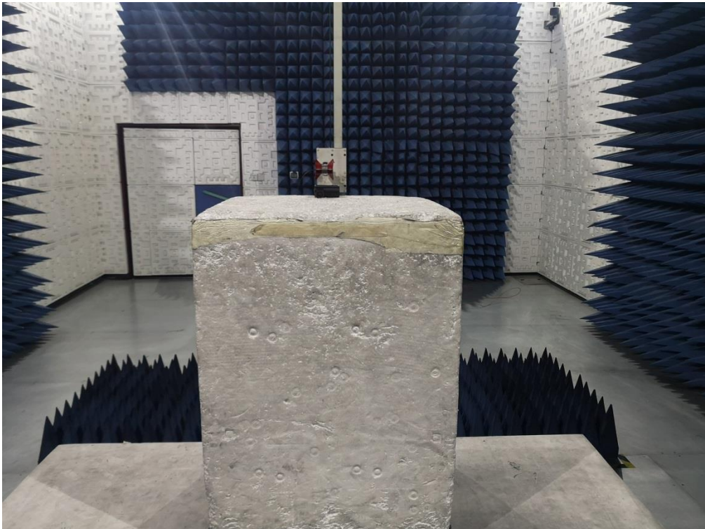
FCC RADIATED EMISSION TEST SETUP ABOVE 1GHZ
