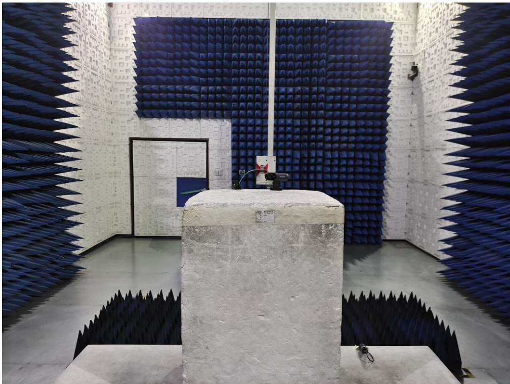
RADIATED EMISSION TEST SETUP ABOVE 1GHZ
